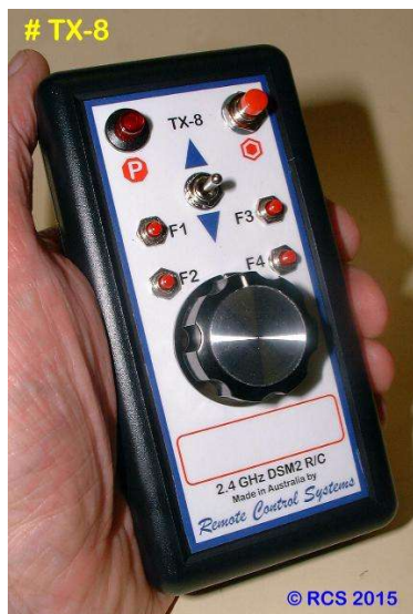
CENTRE OFF LARGE KNOB WITH DÉTENTE FOR 150° CONTROL. EITHER SIDE OF NEUTRAL.
