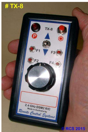
SWITCH FOR DIRECTION SETTING. 300° KNOB FOR LOW OFF CONTROL OF SPEED.
