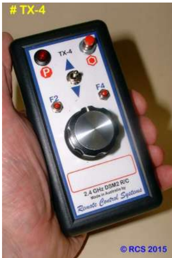
NEUTRAL OFF POSITION OF THE TX-4 WHEN USED FOR "CENTRE OFF" MODE.
