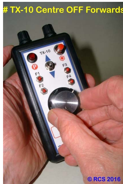
To drive forwards. With the ESC in neutral, twist the knob to the right.
