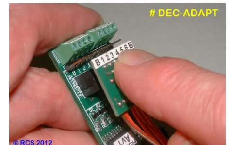
Carefully line up the # SIG-ADAPT pcb with pin #'s 1 - 6 on the # DEC-v3.2 & gently press it home onto the sockets.
