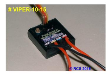
The VIPER ESC's do not have directional constant brightness lightness output controls. Use the RCS # REV-LT to have automatic constant brightness directional lighting.
