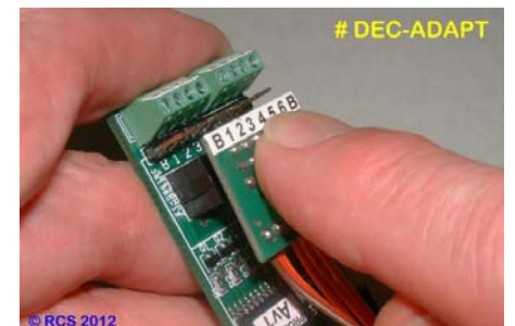
Carefully line up the # DEC-ADAPT pcb with pin #'s 1 - 6 on the # DEC-v3.2 & gently press it home onto the sockets.
