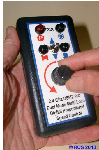
2.4 Rotate Throttle knob from Min to Max & back a couple of times. Pause briefly at each extreme.
