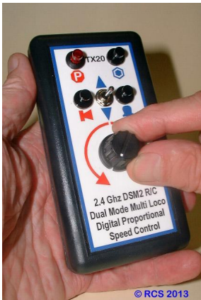
2.1 Turn the TX20 ON. Make sure Throttle knob is set to Min. (i.e. fully CCW).
