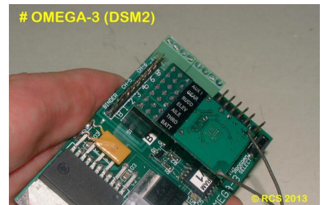
The fit will be tight. Do not force. The BATTERY – BIND terminals must NOT be connected.
