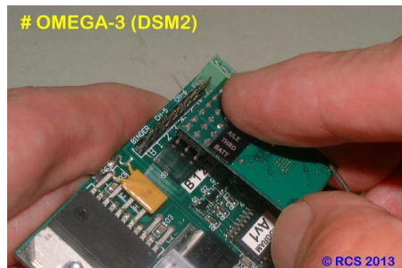
Then gently press RX into socket.
