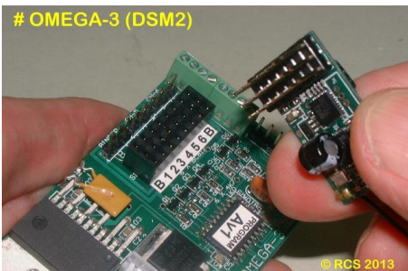
Hold one part in each hand. Carefully line up pins # B – 6. Earlier version # OMEGA-3 shown.
