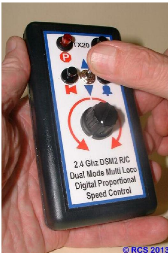
2.3 Move the spring loaded direction switch backwards & forwards full travel a couple of times. Pause briefly each way then let switch go.
