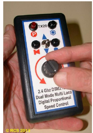
2.4 Rotate Throttle knob from Min to Max & back a couple of times. Pause briefly at each extreme.
