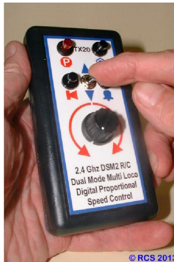
2.3 Move the spring loaded direction switch backwards & forwards full travel a couple of times. Pause briefly each way then let switch go.
