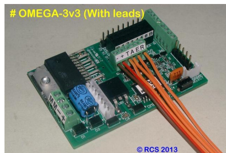
Insert the # ESC-LEADS as follows. T = Throttle. A = Aileron. E = Elevator. R = Rudder.
