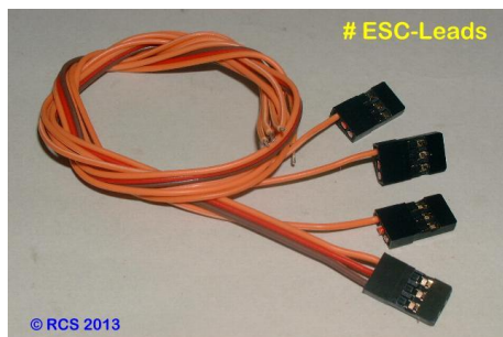
The # ESC-LEADS kit. These connect a non DSM2 RX to the # OMEGA-3v3 ESC.
