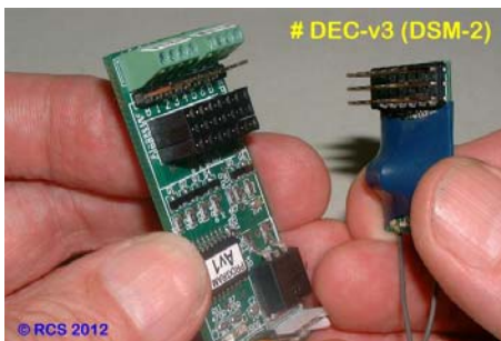
Hold one part in each hand. Carefully line up pins # 1 - 6.
