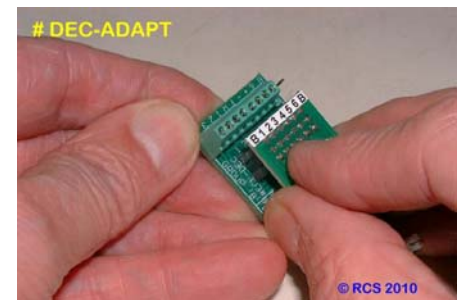
Carefully line up the # DEC-ADAPT pcb with pin #'s 1 - 6 on the # ECL-DEC & gently press it home onto the sockets.
