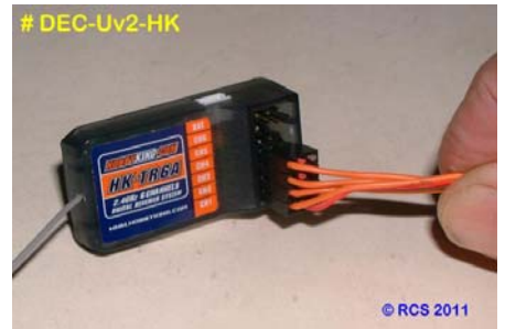
Insert the 1 x 3 way servo cable & four single wire cables into the TR6a RX. Connect as per the chart below.
