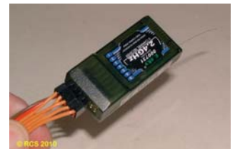
Insert the supplied servo cables into the servo sockets on RX. As per chart BELOW.
