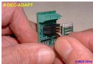
Carefully line up the pins on # DEC-ADAPT with the pins # 1 – 6 on # DEC-U .
