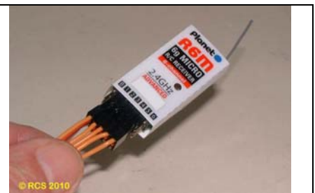
Insert the supplied servo cables into the servo sockets on the # R6M RX. The 3 x wire lead goes to # 1.
