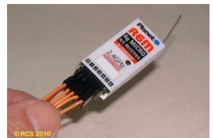
Insert the supplied servo cables into the servo sockets on the # R6M RX. The 3 x wire lead goes to # 1.
