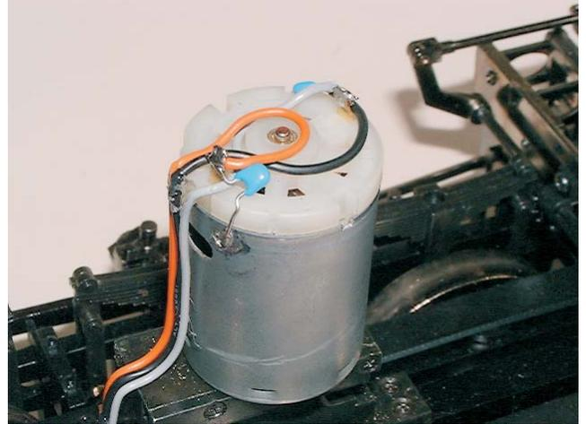
If you are opting for a level #2 or #3 installation remove the wires from the motor and disconnect the in-line plug located in the boiler & discard them. Now feed the supplied Red/Black Tender-Loco harness wires with the smaller "winged" plug into the rear of the loco & then along the top of the chassis up to the motor. Solder the wires to the motor. Black to the front. No motor "Noise" suppression is needed. Ignore caps shown Locate & secure the cable with small dabs of hot
