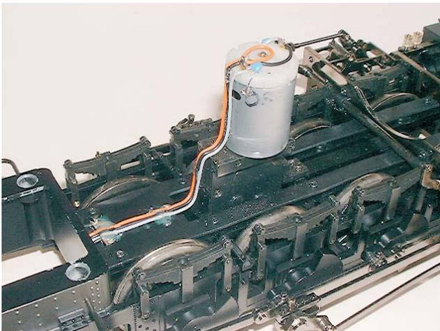
Cut a notch in the underside of the boiler where the motor fits to allow enough room for the cable to clear.
