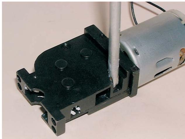
Remove the four screws that hold the gearbox plate on and set the parts aside.
