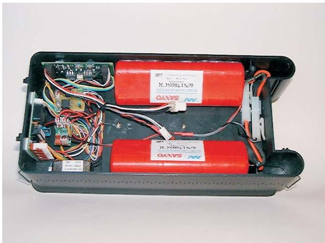
The least expensive type of battery packs to use are 2 x 7.2 twin stick Sub "C" NiCad cells. These are fitted with Tamiya plugs. Because the Bachmann 2-8-0 tender shell is shallower than the 4-6-0 these packs will need to be canted over to fit.
