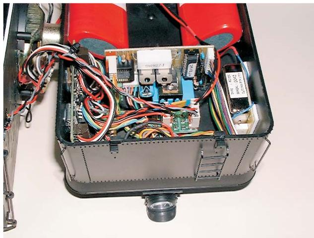
Placement of the older **RCS ESC** system components is shown in the picture above right. Newer systems are smaller allowing different placement. Use a silicone adhesive to secure the parts.
