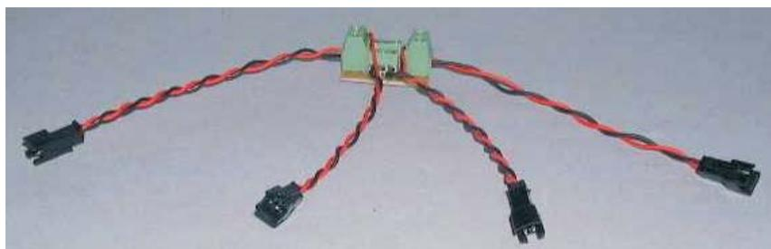
Sample cable with shortened leads to illustrate how the loom is set up.
