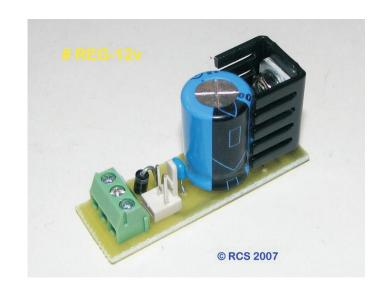
This voltage regulator will be supplied either as 5 or 12 volts. It is designed to power fans or sound systems etc.
