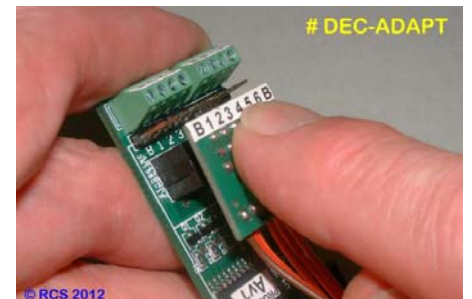
Carefully line up the # DEC-ADAPT pcb with pin #'s 1 - 6 on the # DEC-v3 & gently press it home onto the sockets.
