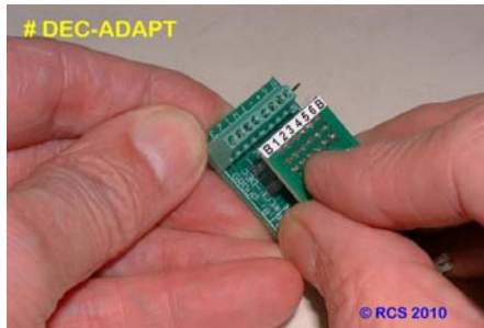
Carefully line up the # DEC-ADAPT pcb with pin #'s 1 - 6 on the # DEC-U & gently press it home onto the sockets.
