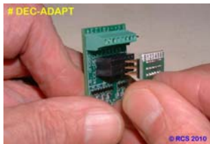
Carefully line up the pins on # DEC-ADAPT with the pins # 1 – 6 on # DEC-U .
