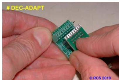
Then gently press the pcb into the sockets.
