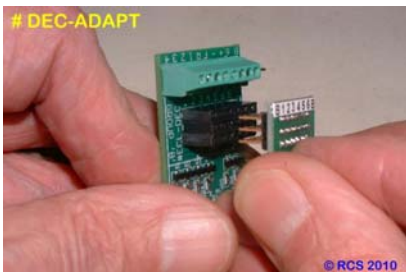
Carefully align pins 1 – 6 of the small # DEC-ADPT kit pcb with the sockets marked 1 – 6.
