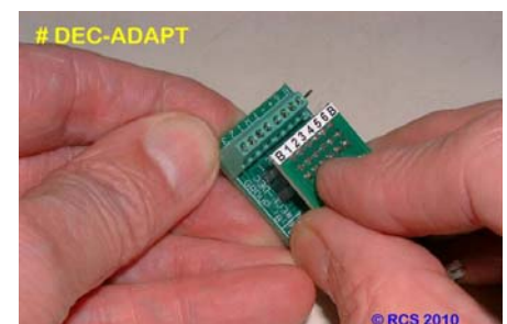
Carefully line up the # DEC-ADAPT pcb with pin #'s 1 - 6 on the # DEC-U & gently press it home onto the sockets.
