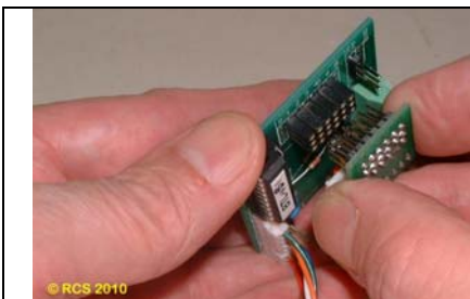
Carefully align pins 1 – 6 of the small # DEC-ADPT kit pcb with the sockets marked 1 – 6.
