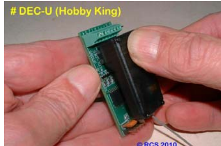
Then gently press onto socket. The fit will be tight. Do not force. The BATTERY – BIND terminals must NOT be connected.
