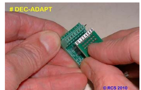
Carefully line up the # DEC-ADAPT kit with pin #'s 1 - 6 on the # DEC-U & gently press it home onto the sockets.
