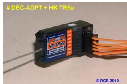
Insert the 1 x 3 way servo cable & four single wire cables into the TR6a RX. The 3 x wire cable goes to # 1 servo output.
