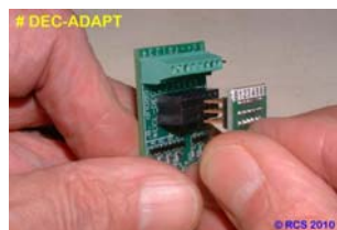
Carefully line up the pins on # DEC-ADAPT with the pins # 1 – 6 on # DEC-U .
